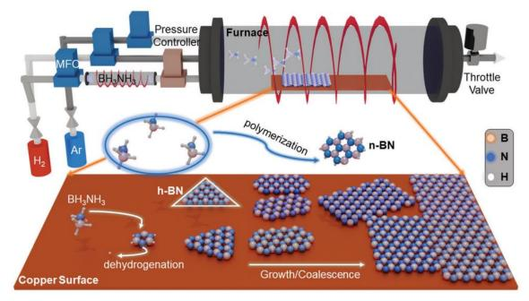
Fig. Schematic illustration of the reactor setup for a true chemical vapor deposition system, along with depiction of the two decomposition pathways leading to growth of the desirable h-BN and undesirable n-BN byproducts.
