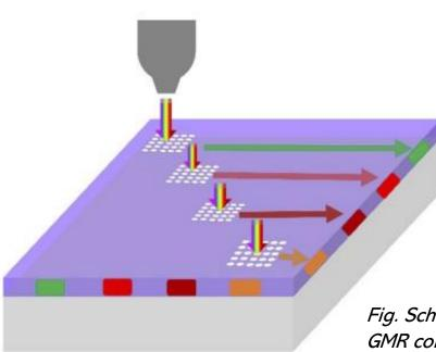
*Fig. Schematic of the on-chip, in-plane GMR colour filters.*
