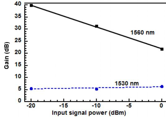
Fig. 3. Gain plotted as a function of input signal power level. The pump power is 7.6 W, and the length of gain fiber is 50 m.
