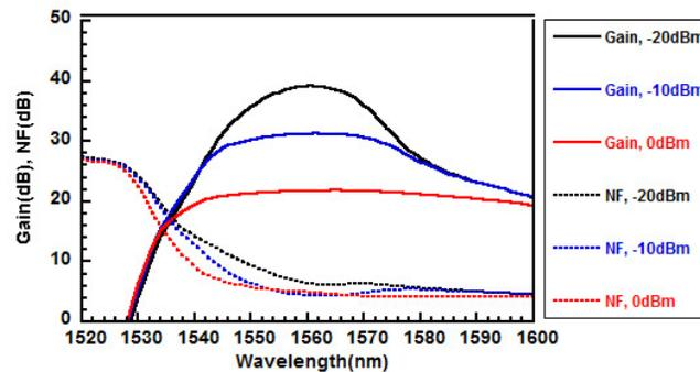
Fig. 2. Gain plotted as a function of wavelength for different signal power level. The pump power was 7.6 W and the length of the fiber was 50 m.
