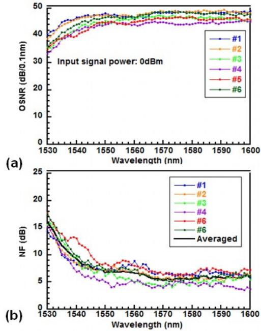
Fig. 7. The measured OSNR (a) and calculated NF (b) plotted a function of wavelength for different cores of the multicore EDF amplifier. The launched pump power was 7.6 W and the input signal power was 0 dBm.
