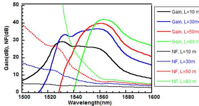
Fig. 1. Gain and noise figure plotted as a function of wavelength for different lengths of doped multicore fiber. Pump power was 7.6 W and input signal power was held at  $-20$  dBm.
