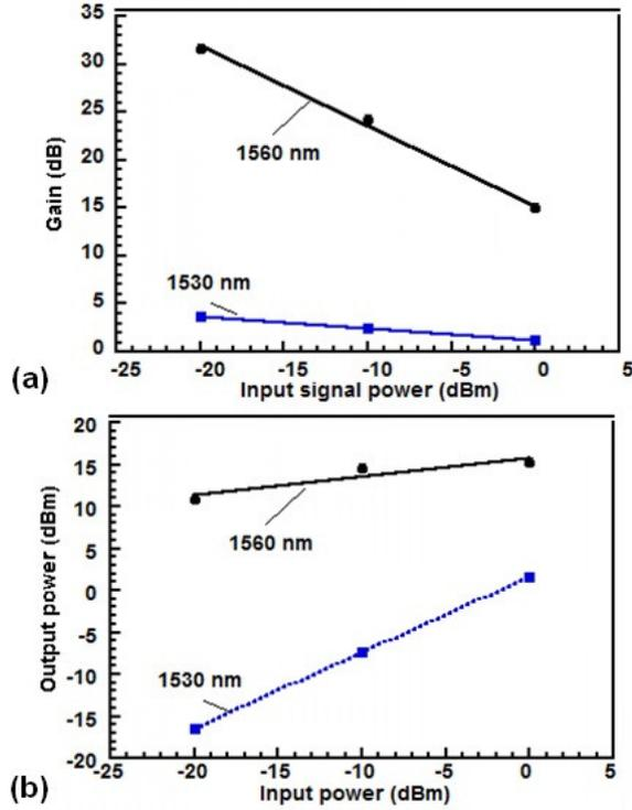
Fig. 6. (a) Measured gain at 1530 and 1560 nm (core #6) plotted as a function of input signal power. (b) Output power plotted as a function of input signal power. The launched pump power was 7.6 W.
