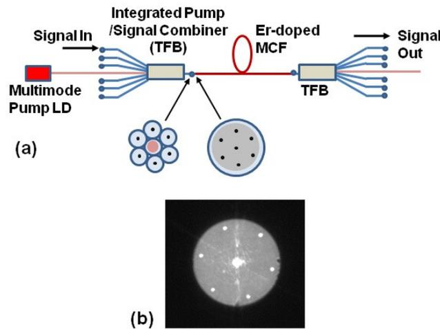
Fig. 4. Schematic of multicore fiber amplifier (a). Photograph of the cross section (with coating removed) of the multicore erbium-doped fiber (b).
