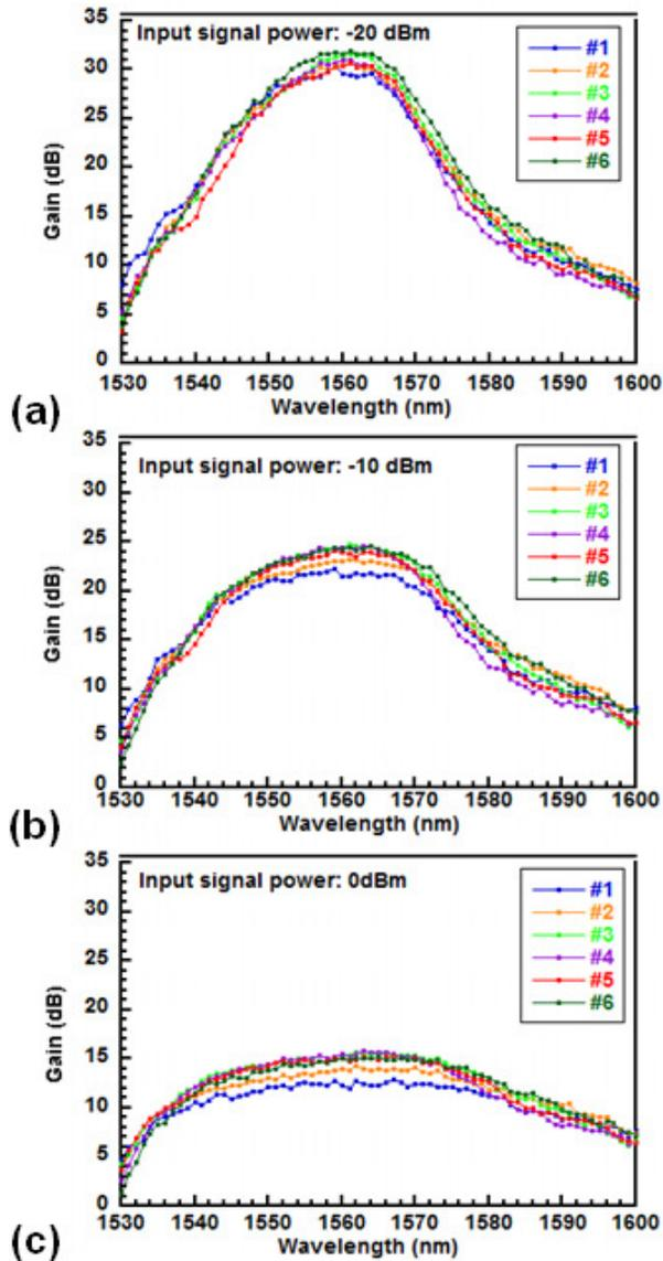
Fig. 5. Net gain measured for different cores of the MC-EDFA. The input power was (a)  $-20$  dBm (b)  $-10$  dBm, (c)  $0$  dBm. Power of pump launched in to the MCF-EDF was  $\sim 7.6$  W.
