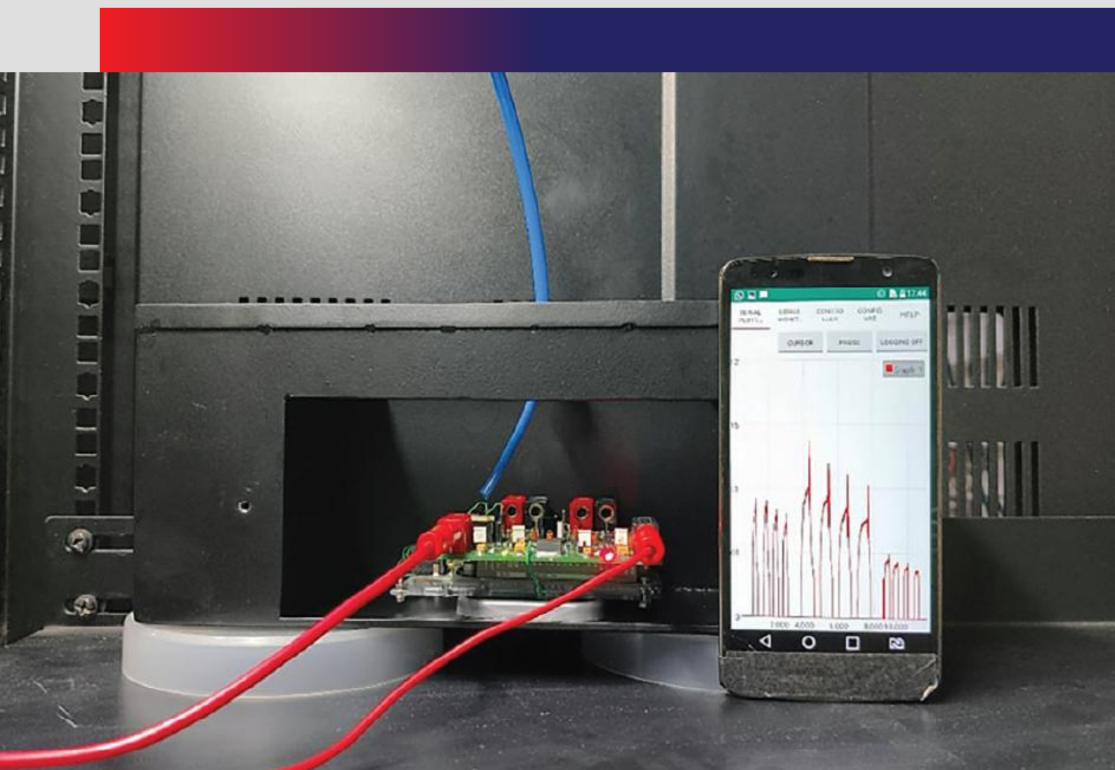
Fig. Real-time \text{SO}_2 leakage detection and monitoring
