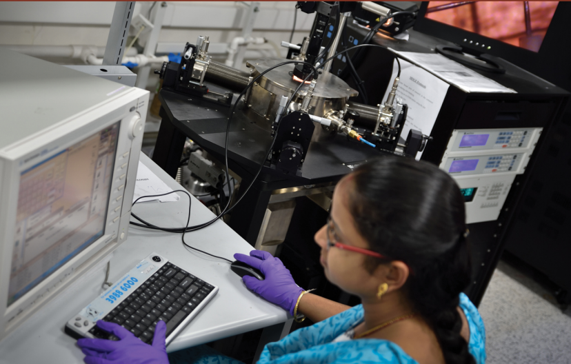
DC Probe Station 4 ▼
